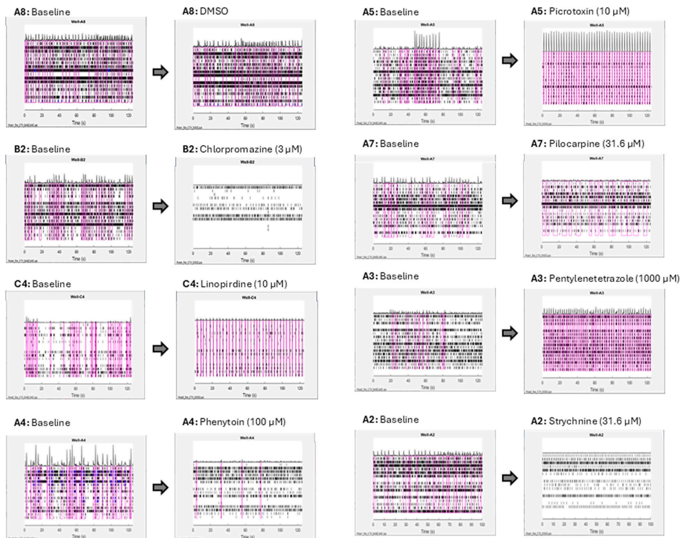
Fig. 2. Example raster plots for rat primary cells grown on MEAs, where the x-axis is the time in seconds and the y-axis rows shows individual neuron firing events (spikes or action potentials). For each pair of plots, the left-hand raster plot is the baseline activity and the right-hand plot shows activity following compound addition.
